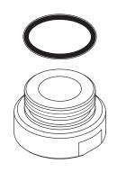
A6256AA Universal filter adaptor. Replaces the Armitage Bioguard outlet to permit attachment of an outlet filter.
