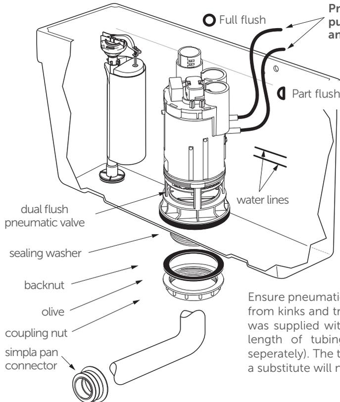
Pneumatic tubes are a tight push fit onto pneumatic valve and flush plate (not shown)
