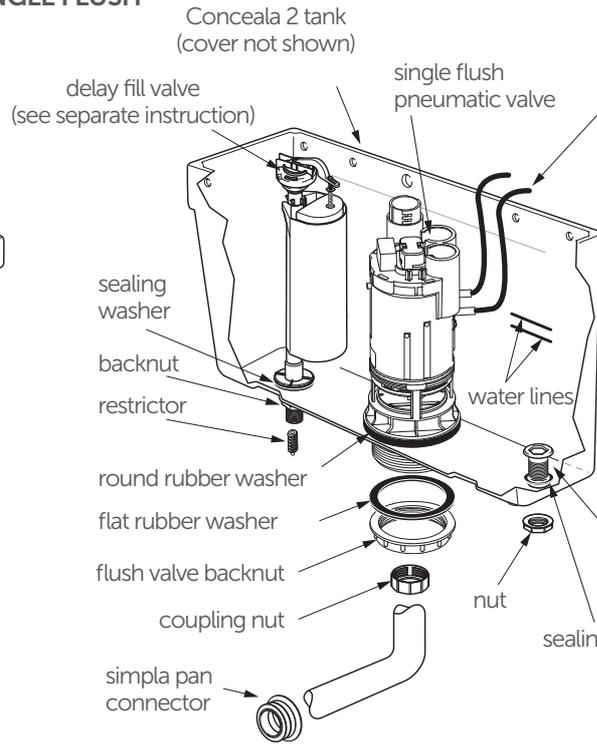
Pneumatic tube is a tight push fit onto pneumatic valve and push button
