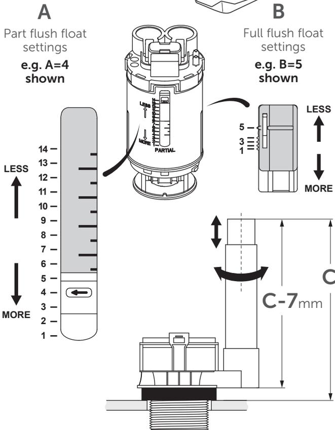
C is the overflow tube height measured from the base of the tank. Subtract 7 if measuring from the base of plastic cage without the seal.
