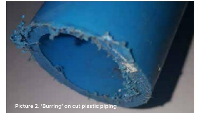
Picture 2. 'Burring' on cut plastic piping
