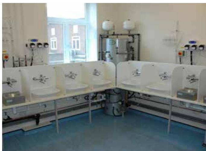
Porton Down test rig - sinks with fast or slow drainage. Image courtesy of PHE, Porton Down
