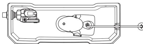
1. Fit the syphon. Check the angle is positioned correctly, towards the fulcrum lever arm assembly location. Ensure the seal is inside the cistern and tighten syphon back nut. The syphon is factory set to 6L.
