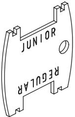
To replace/clean/service the outlet, use the outlet key supplied with the product to unscrew the AV housing. Using the side of the key marked "junior" locate the key into the inner ring of the housing and unscrew. Change the outlet & re-secure the housing with the key, ensuring the seal is in place.
