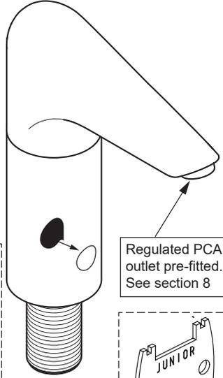
Regulated PCA outlet pre-fitted. See section 8
