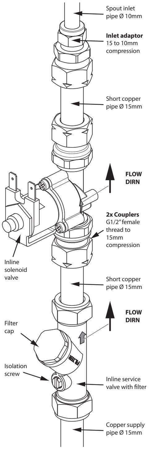
**5. To fit inlet adaptor cont:** Slip the larger compression nut & olive onto a short length of Ø15mm supply pipe. Push the supply pipe into the adaptor up to the shoulder. Slide the olive up to the adaptor & tighten the compression nut with a 24mm A/F spanner. Hold the adaptor steady with a 22mm A/F spanner.
