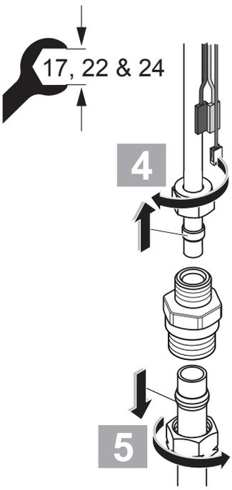
**4. To fit inlet adaptor:** Slip the small compression nut & olive onto the Ø10mm inlet pipe. Push the adaptor onto the inlet pipe up to the shoulder. Slide the olive up to the adaptor & tighten the compression nut (17mm A/F) with an adjustable spanner. Hold the adaptor steady with 22mm A/F spanner.
