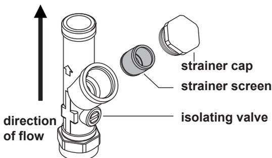
When the isolator screw slot is parallel to the valve body, the valve is open & permits water to flow. To close the valve, rotate the isolator screw 90°.
