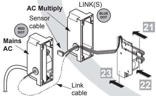
ALTERNATIVELY, the link cable can be routed through the PSU lid as shown in 24, along with the sensor cable.
