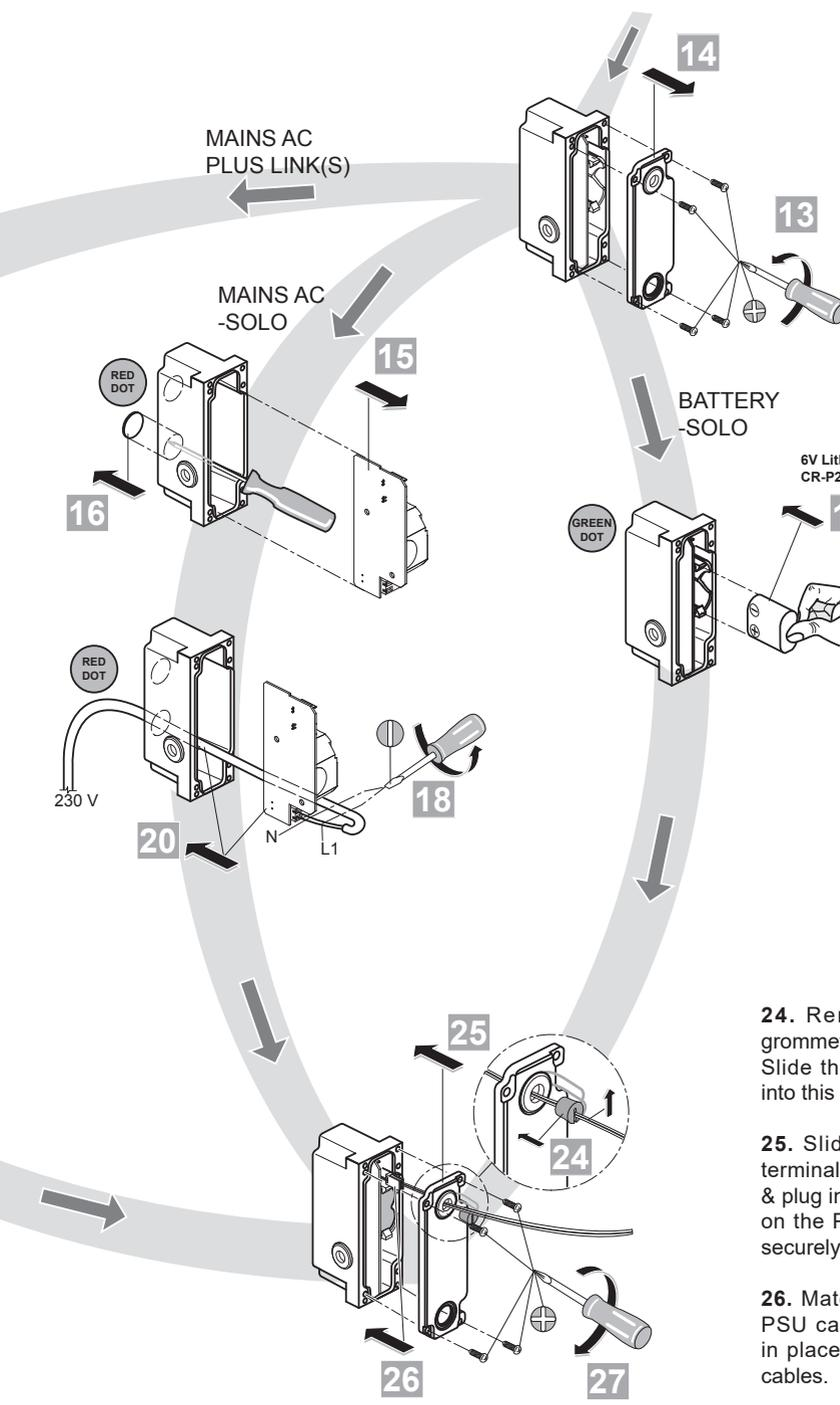
**24.** Remove the pre-split grommet from the PSU lid. Slide the grey sensor cable into this grommet.
