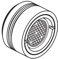
**Outlet cleaning.** On a regular basis the outlet should be inspected & cleaned. To unscrew and remove the outlet, see section 8.
