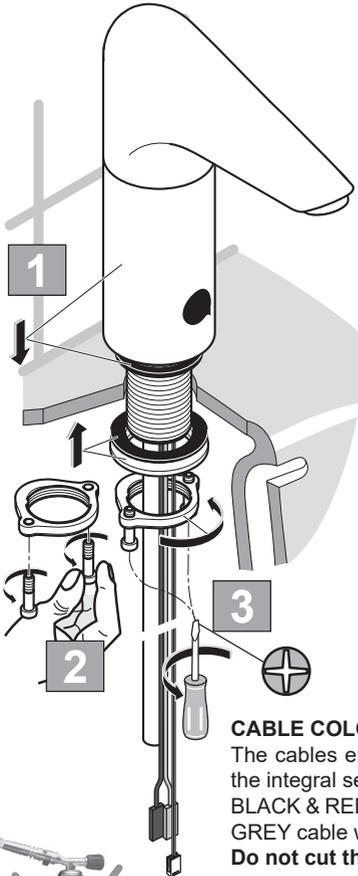
Feed the inlet pipe & cables through basin hole. The cables are protected by the black corrugated plastic tubing (split). Locate the spout tail into the basin hole. Allow the spout to rest on the basin seated on the rubber washer. Refit the corrugated tube if it slips off the cables.
