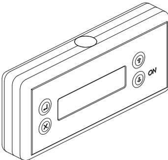
The programming unit should be held pointing towards the sensor at distance of approx. 100mm.
