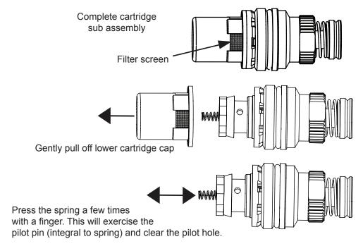
Before reassembling the cartridge cap, make sure that the filter screen is clean (slides out from inside of cap). When reassembling, take care to ensure the spring is straight & locates correctly into the boss at the bottom of the cap moulding.
