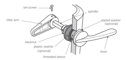
All cistern components must be installed in accordance with UK water regulations. If in doubt a suitably qualified professional should be consulted.
