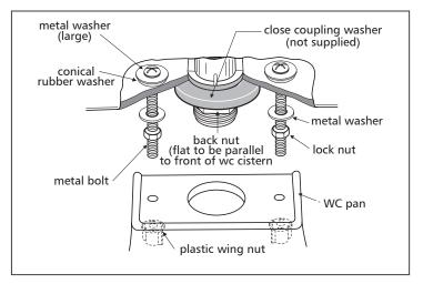
Tighten through bolt assembly using locknut to achieve a watertight seal.
