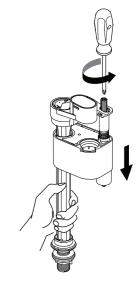
Adjustment of decreasing water level: hold the water inlet body, turn the adjusting screw counterclockwise, and adjust the shut-off cup and the float to the proper position.
